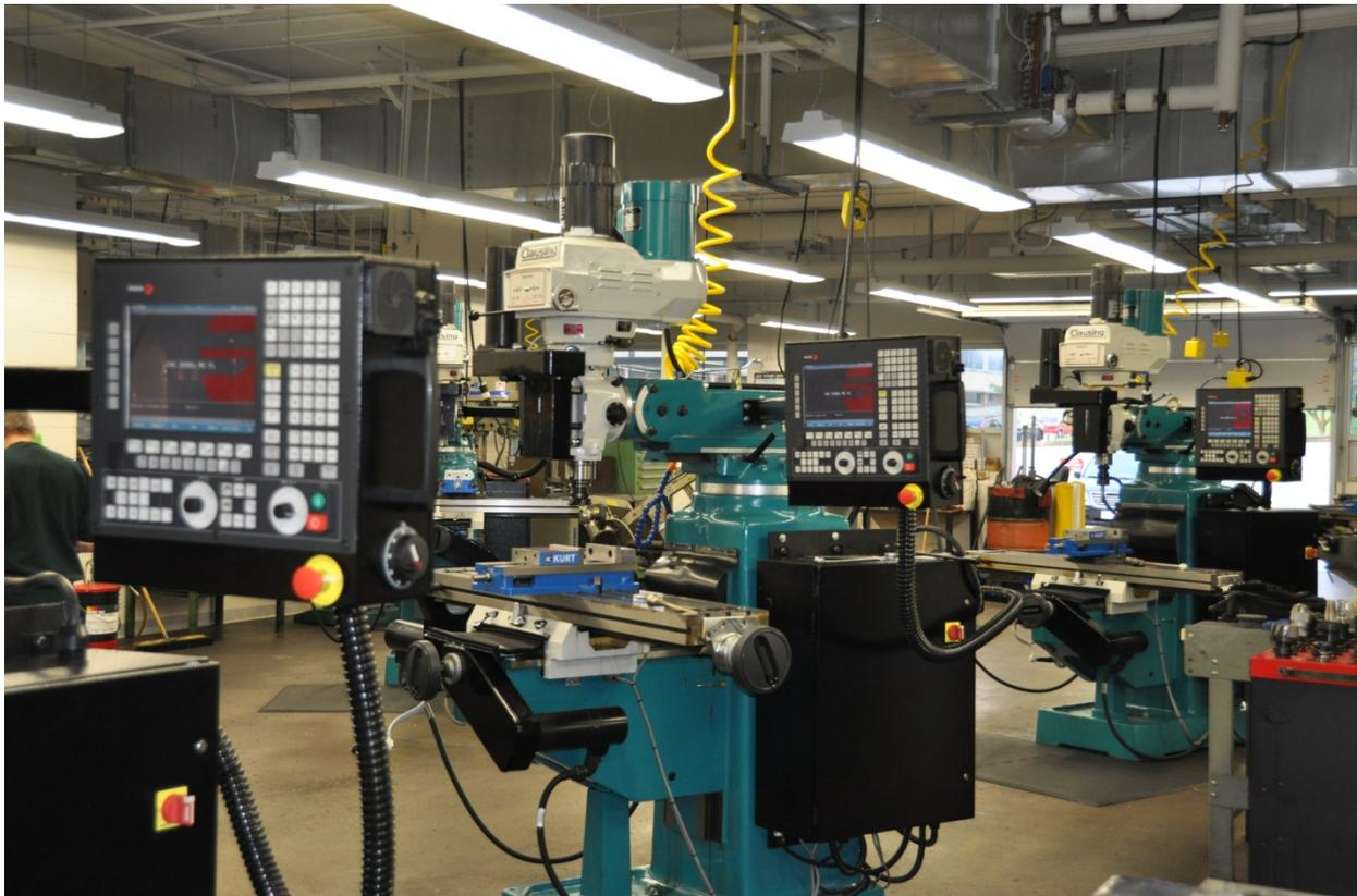
(MATC Shop Floor directly after Iverson & Co delivered 8 Clausing Machines equipped with Fagor 8055 MC Controls)
