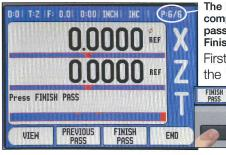
The P:6/6 means you have completed the 5 normal passes and ready to run the Finish and final pass.
