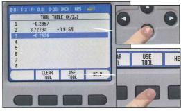
Use up/down arrows to highlight tool and push soft key under **USE TOOL.** You are now ready to start the THREAD CYCLE.
