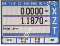
When cursor 'e' centers between the two markers and turns green, engage the Half Nut. For the rest of the passes cursor 'e' will be used to engage the Half Nut. When the TARGET ZONE is reached. disengage the Half Nut.
