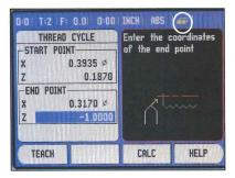
Use down arrow again to highlight Z-axis and input Z-axis end point.
