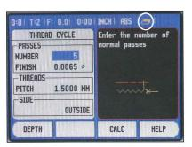
Icon on upper right of screen shows what page you're on This is page one screen of the THREAD CYCLE, where the parameters are set-up. First setting is the START POINT, in the highlighted area input X-axis start point. (Major Diameter)
