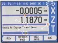
On the first pass only, you will engage the Half Nut (Thread Lever) either by using the thread dial on machine or applying upward pressure on the Half Nut lever until it engages. When you press FIRST PASS, cursor 'a' will move to the right: when the
