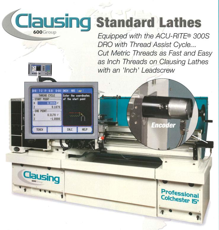
Cutting metric threads on a lathe with an 'inch' leadscrew is difficult and time consuming, requiring a more experienced operator...
