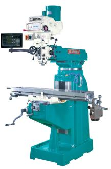
A line of affordable heavy-duty precision CNC knee mills with a wide range of 2 or 3 axes CNC control options and features found only on higher priced machines. Clausing CNC mills can be operated as manual machines with DRO, semi-automatic or full CNC operation.
