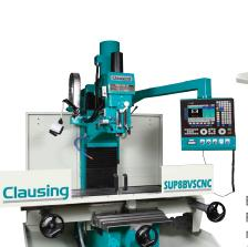
Extra Heavy-duty CNC Bed Mills with Real Cutting Power. Full 3 axis CNC mills available with FAGOR 8055i or ACU-RITE MILLPWR CNC controls. Up to 7.5 Hp spindle drive, 16.75" x 62" table, 2000 lbs. table load.
