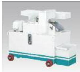
*Coolant System with Magnetic Separator*
