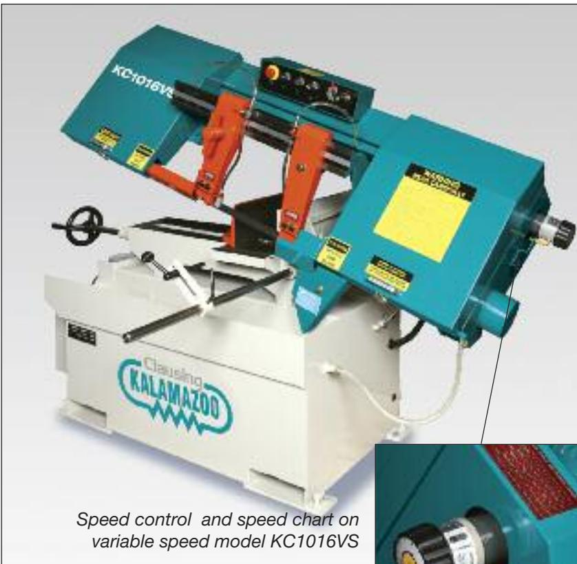
Speed control and speed chart on variable speed model KC1016VS
