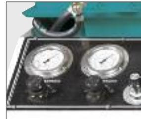
Hydraulic pressure gauges are mounted in the control panel. This lets the operator easily adjust the blade cutting pressure and on models equipped with a hydraulic vise will let the operator adjust hydraulic vise grip pressure.
