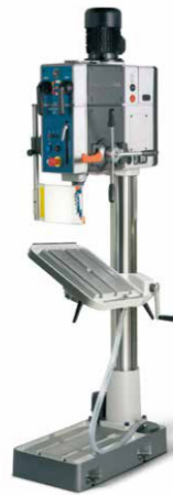
With optional rotating/ tilting table (MGI)
