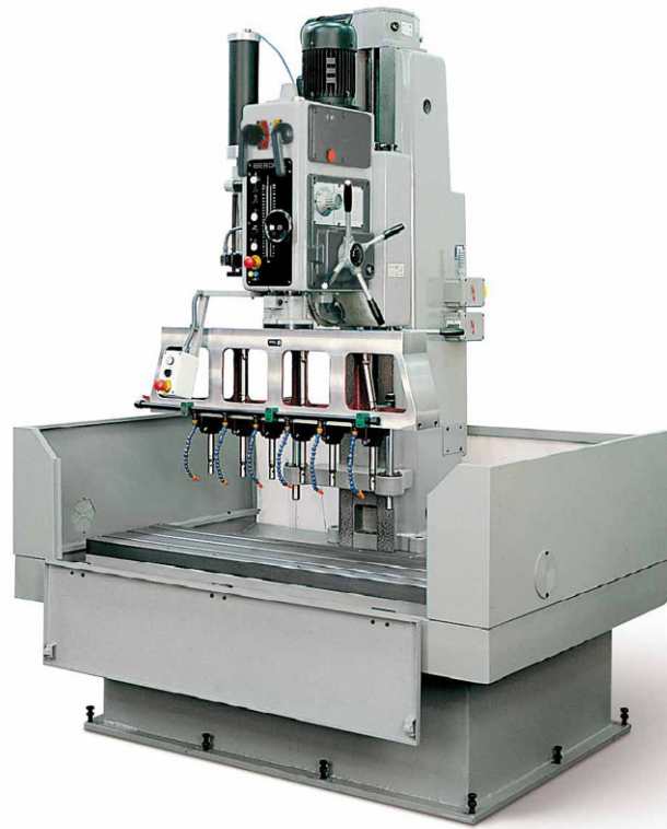
BP50 with extra large table of 400 x 1500 mm for the drilling of rods using a multi-spindle drilling head arranged in a line.
