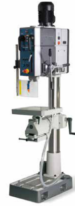
With optional reversible tilting table (MGM)
