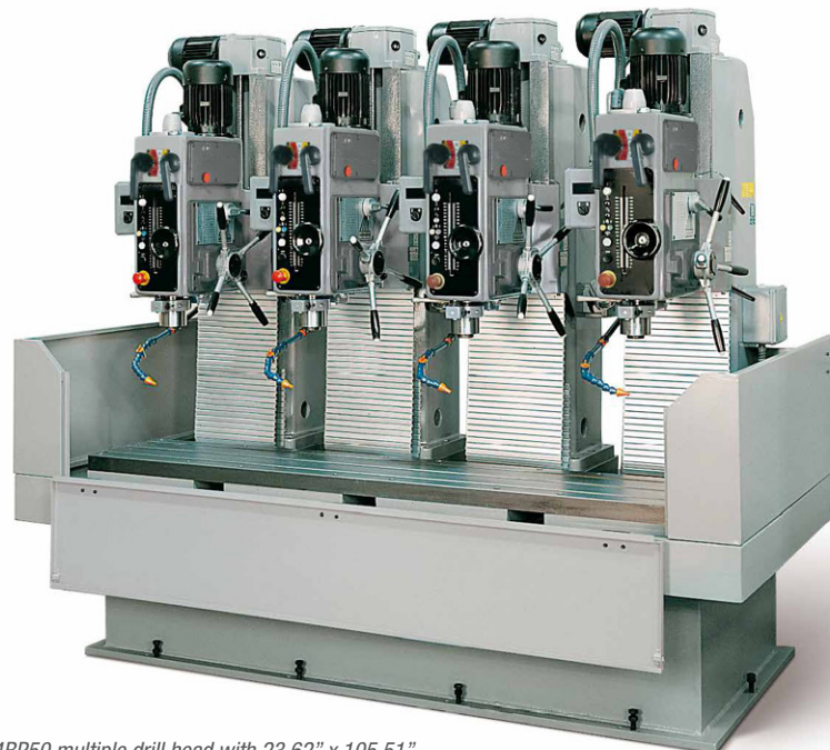
4BP50 multiple drill head with 23.62" x 105.51"
